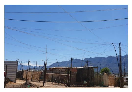
The maintenance of the electrical network remains a major challenge especially with regards to illegal connections which result in unplanned interruptions as networks becomes overloaded.
