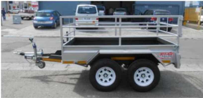
.4M x 1.5M DOUBLE AXLE 2700/3500KG GVM 195/14" TYRES & RIMS GALV/PAINTED
